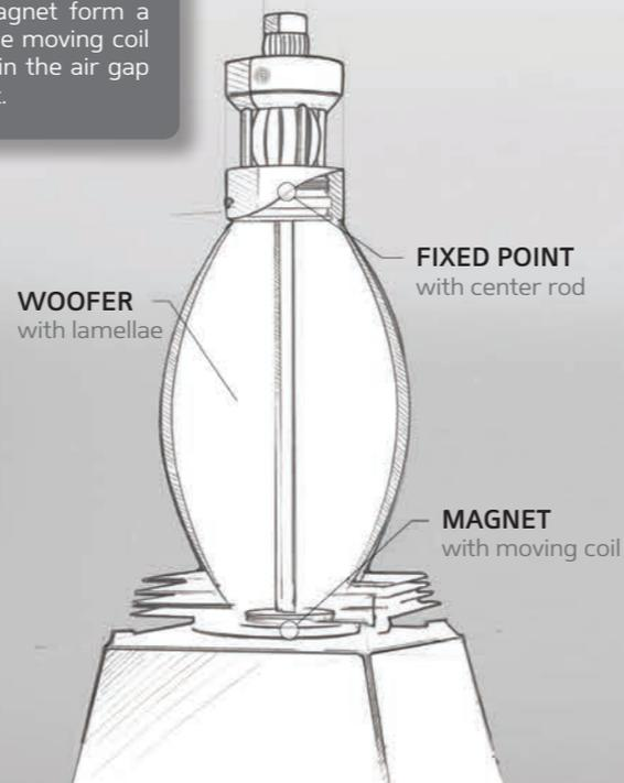
**3** The musical signal, still electrical at this stage, is sent from an amplifier to the speaker. Electricity passes through the moving coil, and the resulting magnetic field allows the coil to move up and down in the air gap of the magnet.
